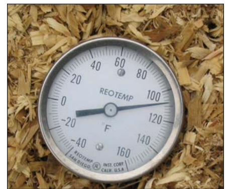
Figure 6. Example of an analog thermometer. Note that this pile needs to be heated up.
