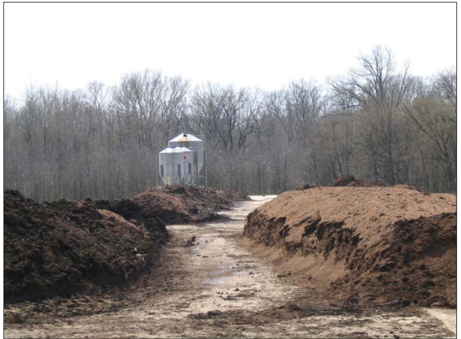
Figure 4. Open windrow composting system.
