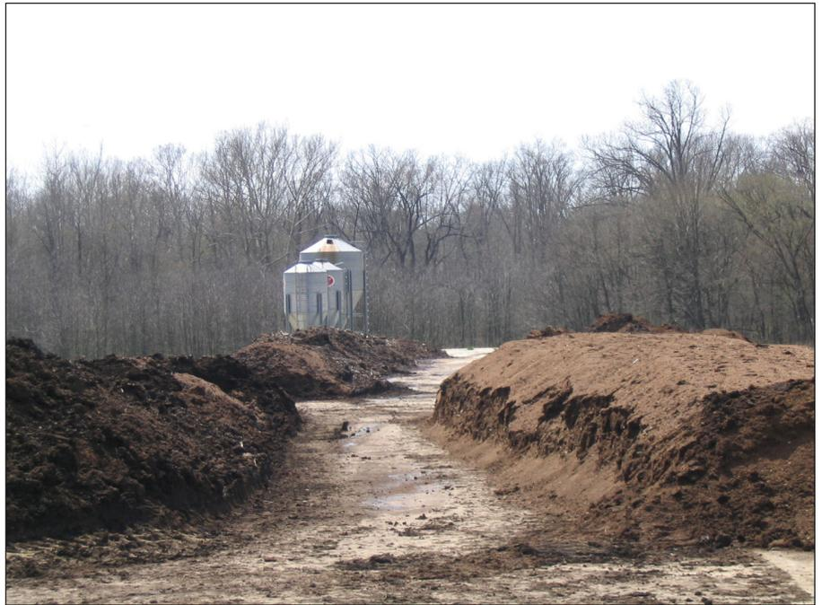
**Figure 4.** Open windrow composting system.
