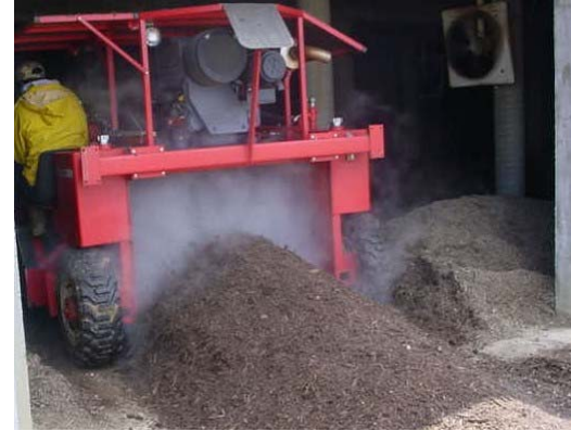
The O'Bryans' new composting machine mixes hog manure with wood chips to create an environmentally-friendly fertilizer.
